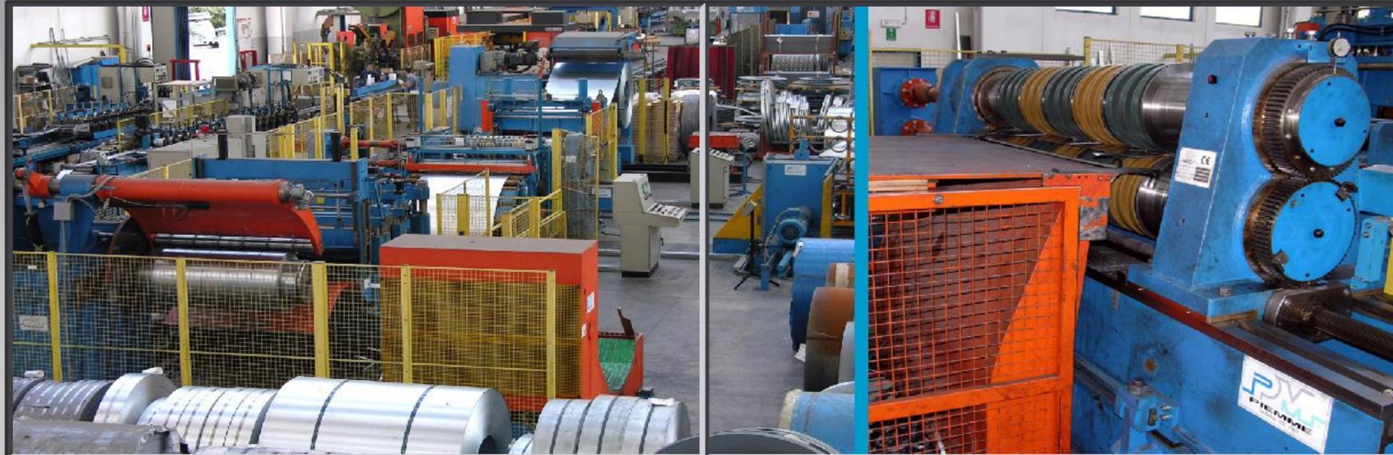
View of line and detail of shear w. circular blade
