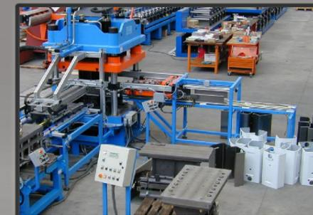
Detail hydraulic press and unloading rolls
