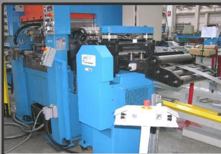
Straightener feeder and press
