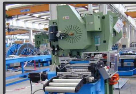
Photovoltaic profile punching
