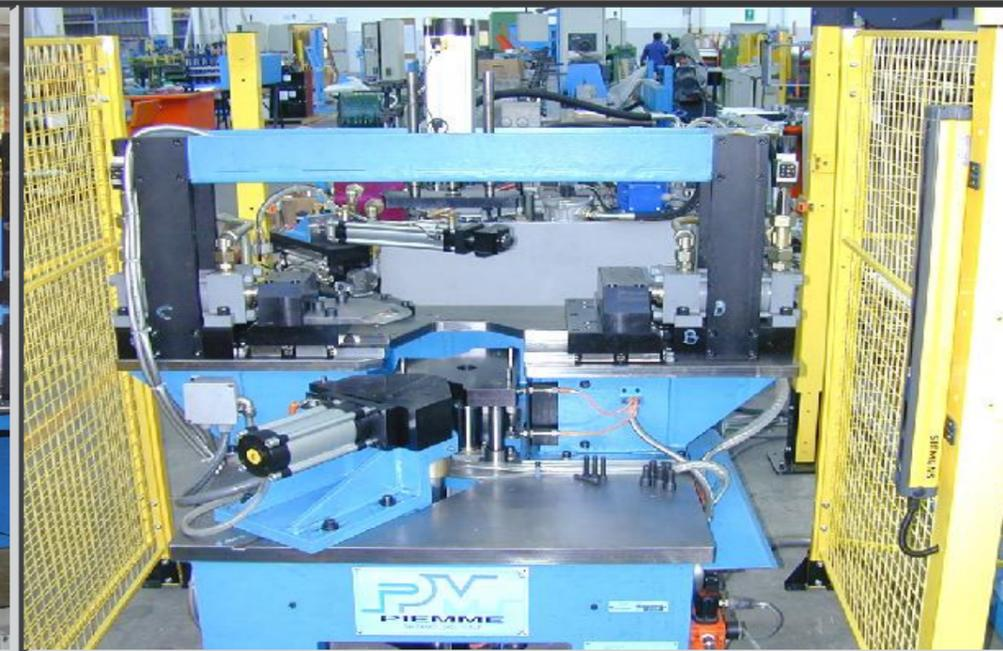
Seaming unit for elbow joints
