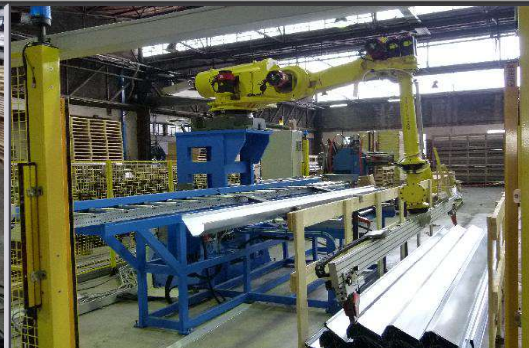
Unloading and stacking robot
